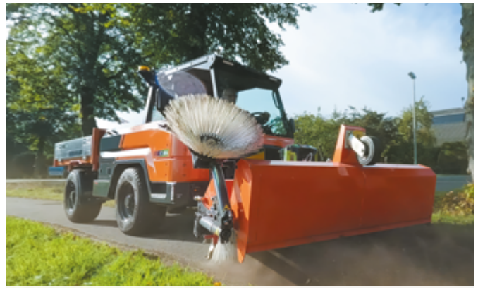
bema Sweezy® 580 Dual E with collection container in the proven Dual system, in this case free sweeping with an open collection container
