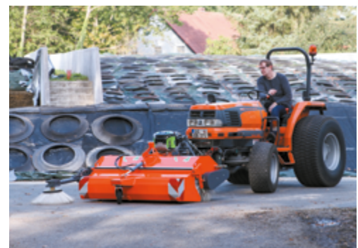
bema Sweezy® 580 Dual E attached to a compact tractor
