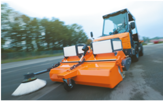
bema Sweezy® 580 Dual E equipped with a mechanically driven rotary side brush and a water spray unit with 2 x 64 Liter water tanks
