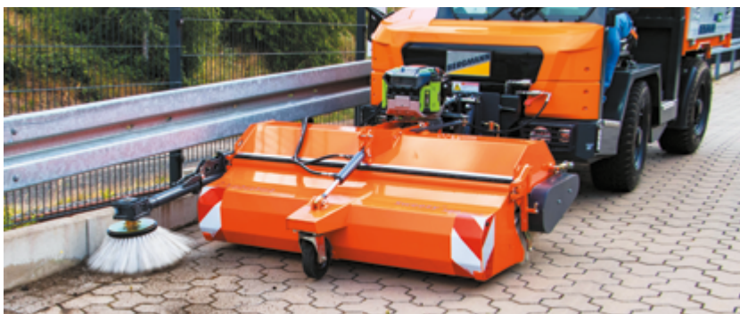
bema Sweezy® 580 Dual E with mechanically driven rotary side brush attached to an e-dumper
