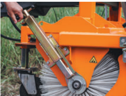
Stepless spindle adjustment of the main brush
